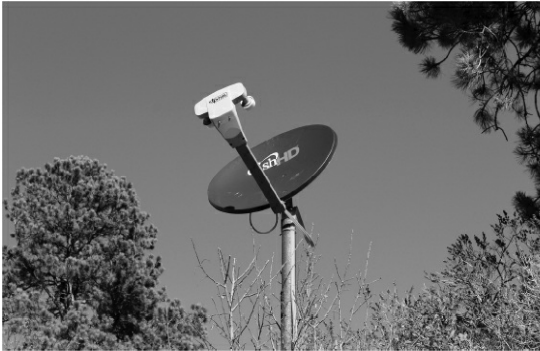
FIGURE 6-11 A typical dish antenna equipped for satellite TV reception and satellite Internet access. It measures about two feet (60 to 70 centimeters) in diameter.
