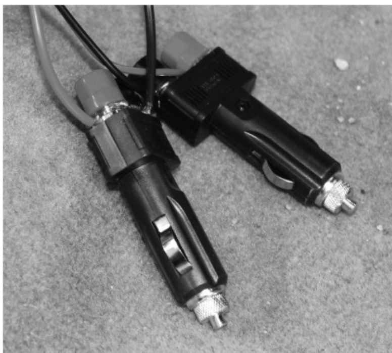
FIGURE 5-11 Power plugs for the radios, with lighter adapters on the ends. The power cords contain separate fuses to protect the radios and the vehicle's electrical system.
