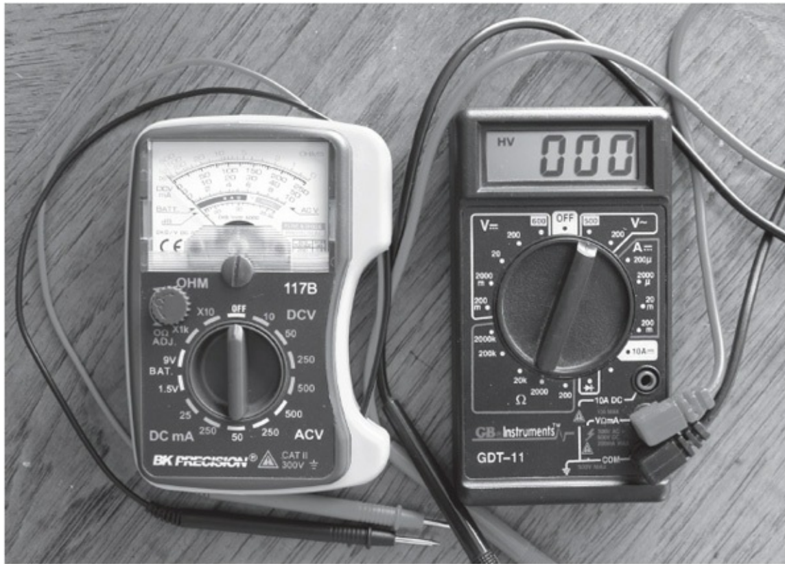
FIGURE 2-10 At left, an analog multimeter. At right, a digital multimeter.
