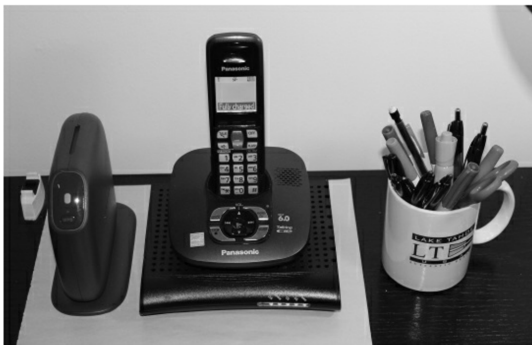
FIGURE 6-9 A cable modem, a cell-phone base unit, and a wireless router. Note the cup with the writing instruments for size comparison.
