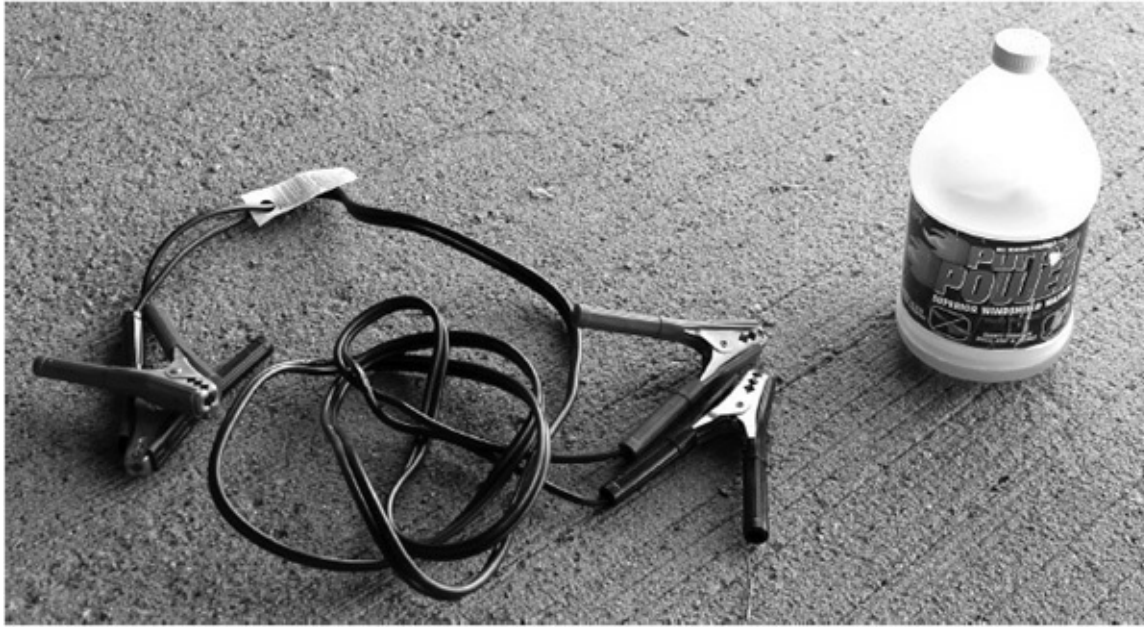
FIGURE 5-2 A pair of jumper cables, roughly 6 feet (2 meters) long, with a gallon jug of washer fluid for size comparison. Note the large clips on the ends.
