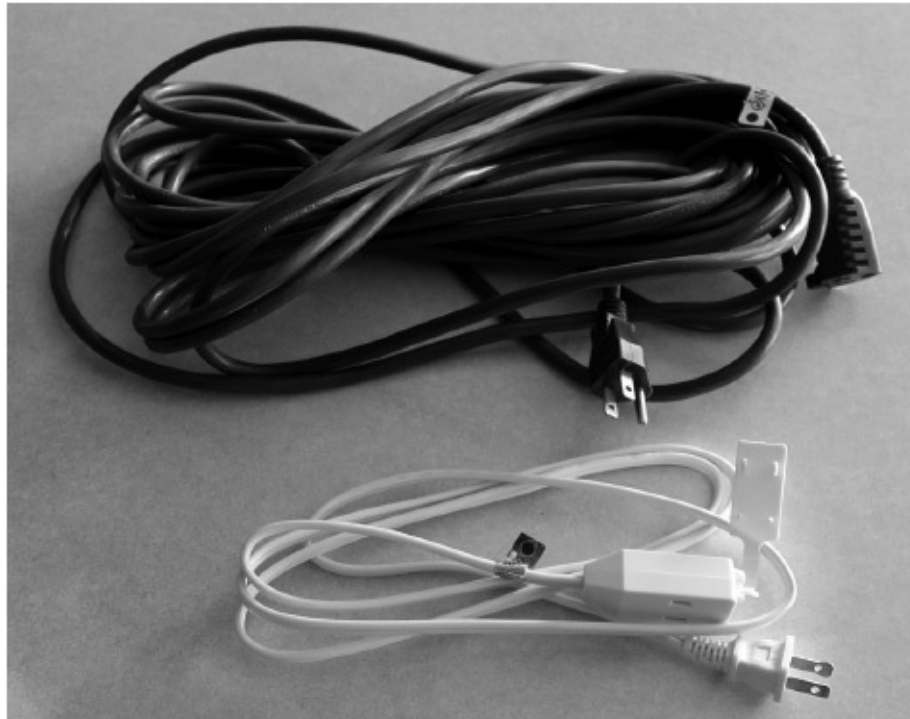
FIGURE 3-8 A 40-foot, three-wire extension cord for indoor/outdoor use, and a 6-foot, two-wire extension cord with three outlets for indoor use. Both cords are rated at 15 A.
