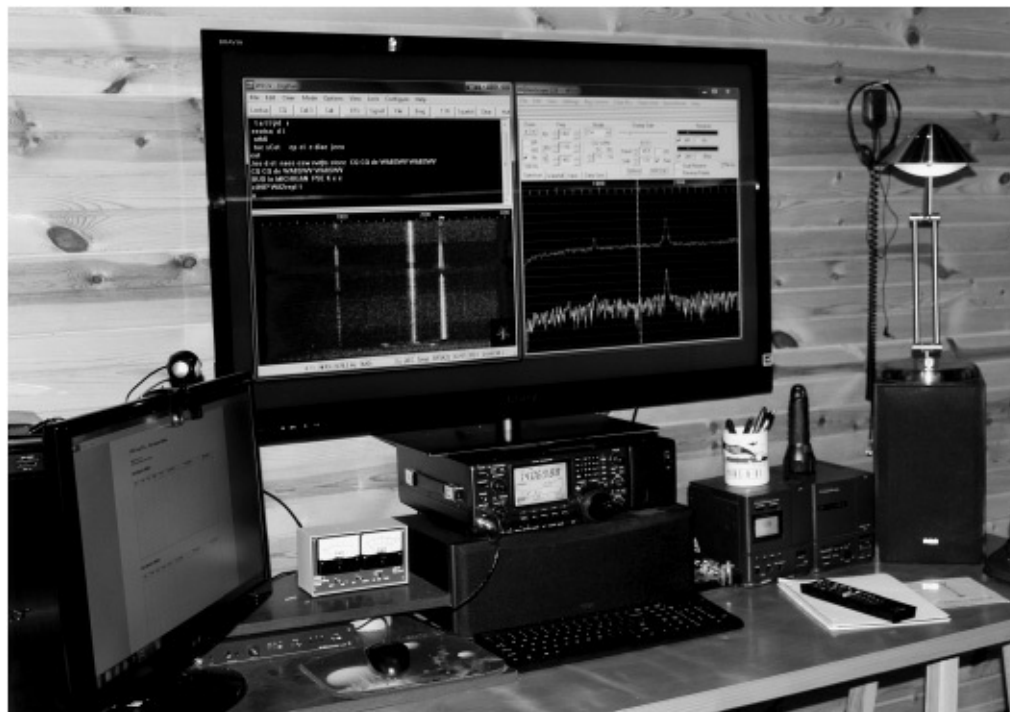
FIGURE 8-11 The author’s amateur radio station including a transceiver, Internet-ready computer, interface for digital radio communications, power meter, hi-fi audio system for big sound, and two displays, one of which is a flat-screen TV set.
