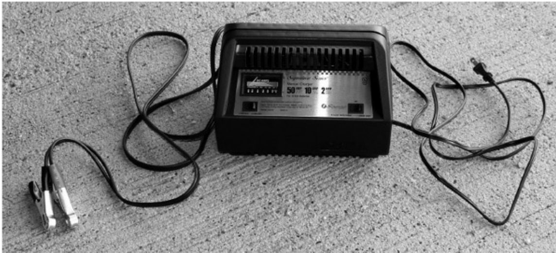
FIGURE 5-4 An “outboard” automotive battery charger with two different current settings. It’s a little smaller than the battery itself (and a lot lighter).
