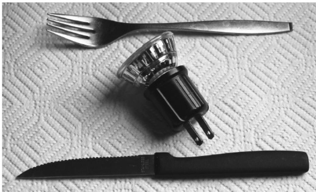
FIGURE 3-7 You can assemble an outlet tester with a standard plug-in bulb socket and a light-emitting-diode (LED) lamp.
