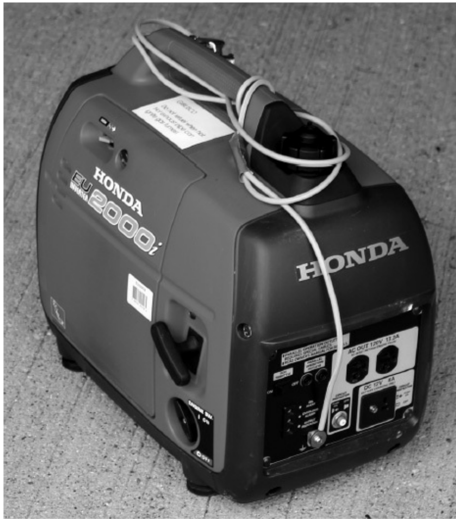
FIGURE 4-1 A portable gasoline-fueled generator, capable of providing up to 2 kW of clean sine-wave AC power at 117 V RMS. The tied-up cord is the ground wire.
