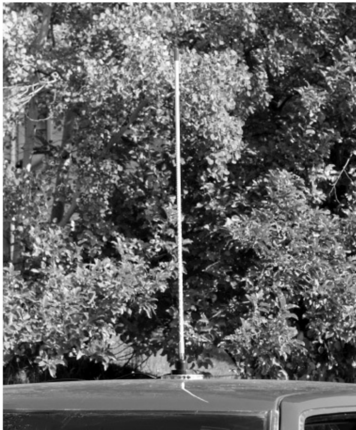
FIGURE 5-12 A CB mobile radio antenna attached to the roof of a pickup truck with a magnetic mount.
