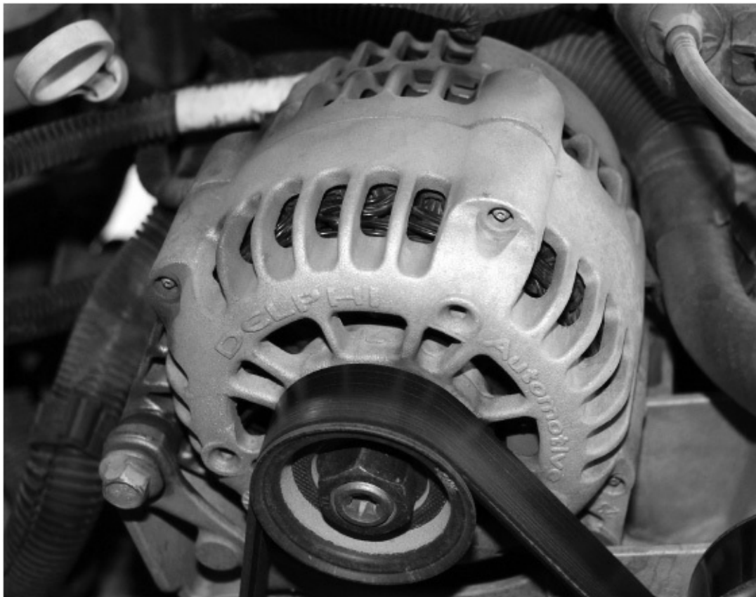
FIGURE 5-5 The alternator looks something like a motor, and is usually located under the hood next to the engine.
