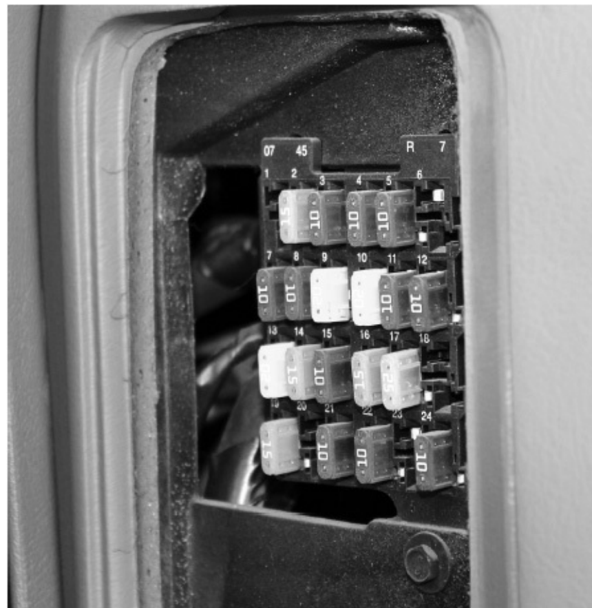
FIGURE 5-9 Fuse box in a typical motor vehicle with the protective panel removed. In this case (a 2003 Chevy S-10 pickup), the fuses are accessible only with the driver’s side door open.
